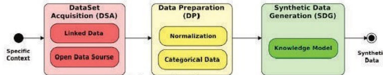
FIG. 1: SYNTHETIC DATA GENERATION ARCHITECTURE
